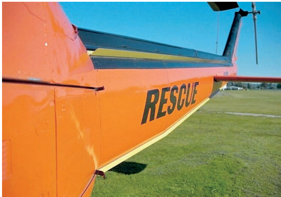
BLR's Bell 212 (opposite) during December 2007 baseline testing in an unmodified configuration at Leadville, Colo. as part of the STC approval process. BLR's strakes (above on a different aircraft) are simple, small, lightweight fences attached to the side of the tailboom (see photo) to change the flow of air around the tailboom for better stability and control.
