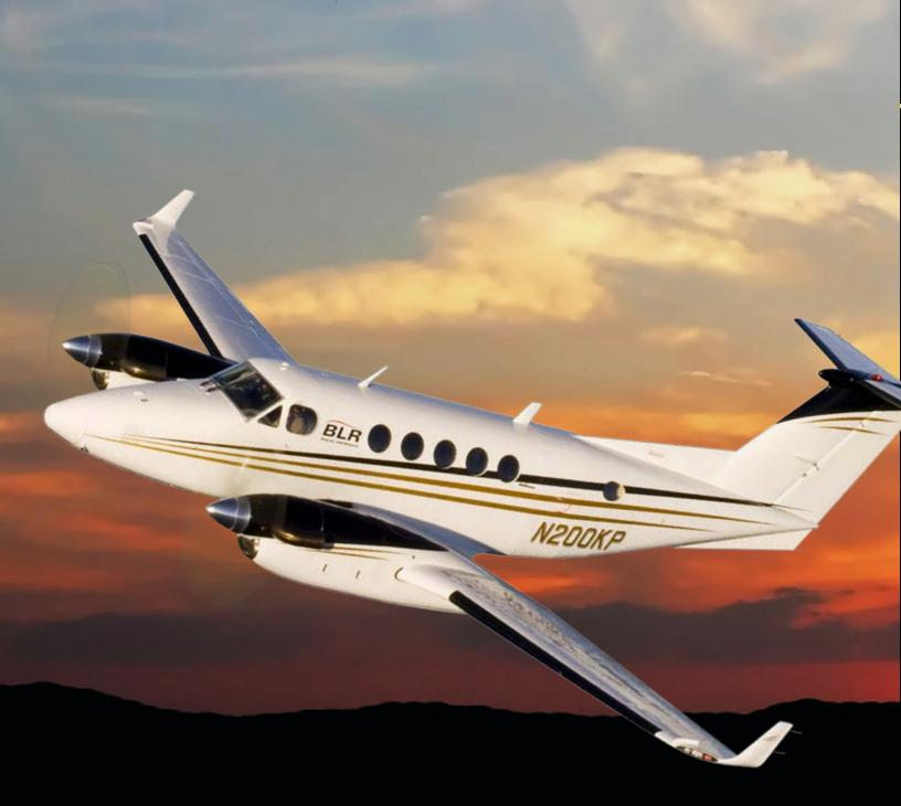
In addition to the King Air 200, above, Winglets are also available for King Air 90s and 300s. In fact, BLR Winglets are standard on all new factory Hawker Beechcraft King Air 90 GTx aircraft.
