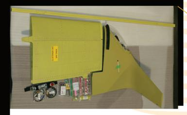
BLR's Winglet System will increase the total wingspan by 3' 5"
